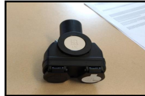
Temporary solution: Distribution adaptor
